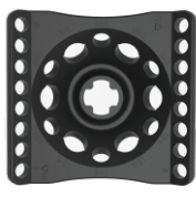
Mini-A-3复合转头 1.5ml×6孔+0.5ml×6孔 +0.2ml×8孔×2排 4000rpm/912×g 7000rpm/2793×g
