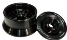
16R A-1(2)角式转头 1.5/2ml×18孔 16000rpm/19550×g
